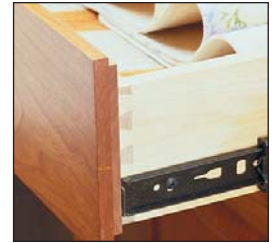
The drawer boxes feature \frac{1}{2} " birch sides joined at the front and back with half-blind dovetails
