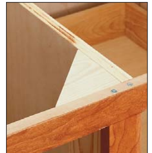
A single stile and a 3/4"-thick plywood divider panel separate compartments in the large base unit.
